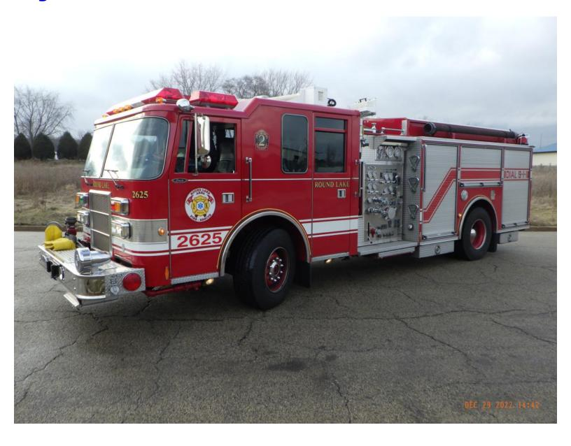
Engine 2625 is a 1998 Pierce fire engine and was built by Pierce Manufacturing in Appleton, WI. It carries six firefighters, has an 500 gallon water tank and can pump 1,250 gallons per minute.
