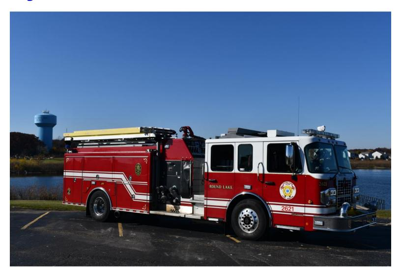
Engine 2621 is a 2015 Spartan chassis and was built by Custom Fab & Body in Marion, WI. It carries four firefighters, has an 800 gallon water tank and can pump 1,250 gallons per minute.
